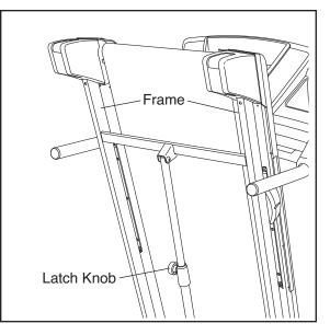
2. Hold the metal frame firmly with both hands and lower it to the floor. CAUTION: Do not grip only the plastic foot rails or drop the frame to the floor. Bend your legs and keep your back straight.
